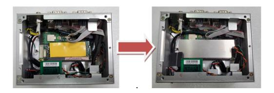
Step 7 Put the bottom cover back and fasten all of screws.
