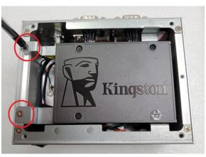
Step 6 Put the bottom cover back and fasten all of screws.
