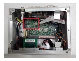
Step 4 Insert the M.2 WiFi module firmly and fasten the screw.
