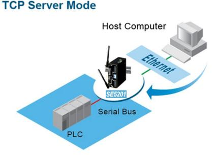
Figure 5.2 SE5201 is set as a TCP Server Link Mode
