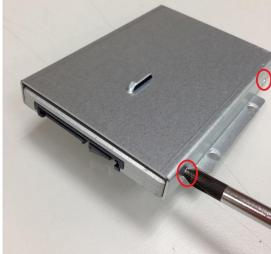
Step 4 Put the HDD bracket on the cover and use 4pcs screws to fix tightly. Takes the
