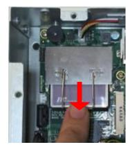
Note: Unlock the CF card from the socket and pull out the CF card when taking out CF card.
