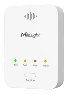
GS101 is a LoRaWAN<sup>®</sup> residential gas detector to detect the natural gas leak and send alarms. When the concentration caused by gas leak reaches the preset threshold, the detector will trigger both LED light alarm and buzzer sound alarm, it also supports controlling outputs to close the gas valve and open the vent fans to prevent potential accidents.
